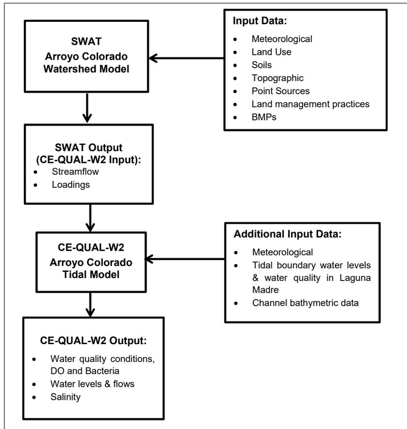
Figure 9.1. Schematic of modeling system
